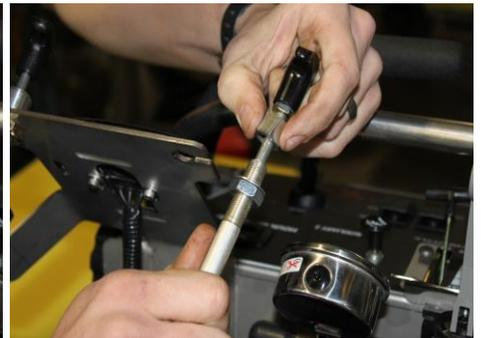
(pull cable down and out to remove)
