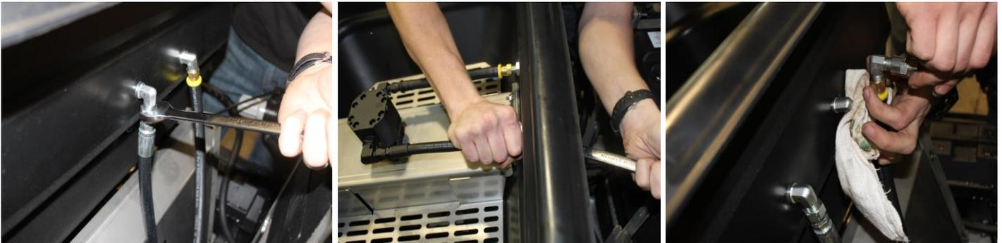
(wrench to loosen rear Hopper fittings) (grab inner hoses to help secure removal) (use rag to catch any runoff fluid)
