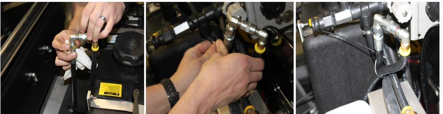
(Connect Hydraulic lines on unit) (locate a good secure area to mount) (secure hose with the Foam Marker hose)
