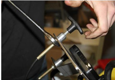
(loosen nut on Diffuser Cable)
