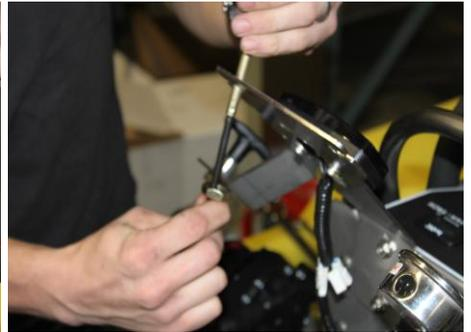
(slide cable out of the Hopper Bracket)
