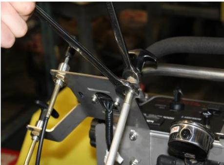
(loosen nuts on cable)
