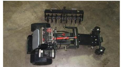
Once the traction unit is free of any attachments (in the under carriage area), drive the aerator traction unit to the rear of the De-Thatch Rake attachment (*pictured below*). Position the rear wheel that is next to the De-Thatch Rake approximately to the middle of the rear end. Turn the front of the unit to position the aerator traction unit over the De-Thatch Rake (*pictured below*) and turn off the engine.
